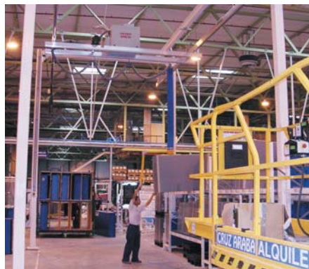
Suspension track system with free-standing portal construction. Work area: 22.000 x 5.000 mm
