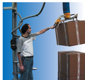
Angle extension: For stacking loads on high levels.
