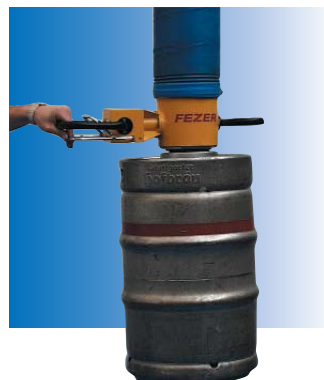
VacuPowerlift VPL with single suction foot SFE 250V for the transport of barrels with a smooth surface.
