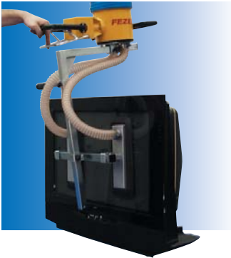
VacuPowerlift VPL with special suction foot for the transport of TV sets.
