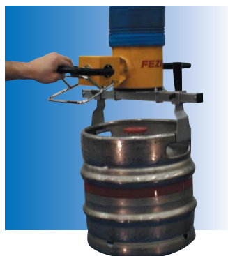
VacuPowerlift VPL with special suction foot for the mechanical transport of drums with grip straps.
