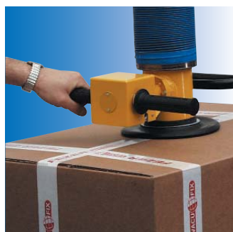
Control unit with turning lever. The tube is lifted and lowered by turning the lever forwards and backwards.
