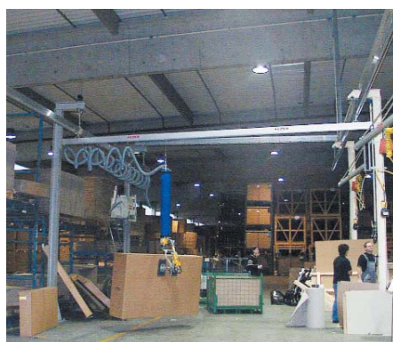
Suspension track system with free-standing portal construction. Work area: 10.000 x 4.000 mm
