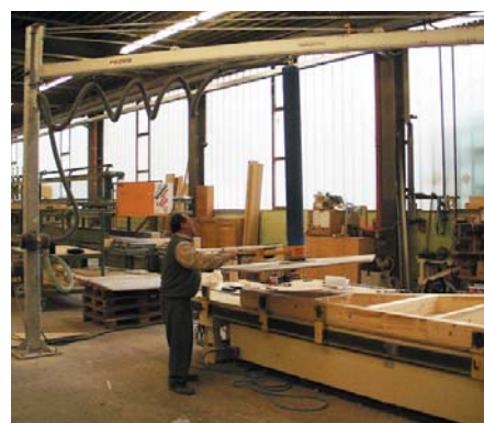
Column slewing jib SSK 160-6.000 for loads of up to 80 kgs
