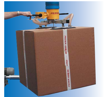
VacuPowerlift VPL with double suction foot SFD 120x320 for glued, strapped or open boxes.
