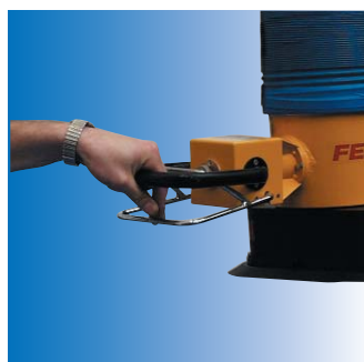
Control unit with tilting lever. The tube is lifted and lowered by pushing the lever upwards and downwards.
