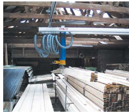
Suspension track system with beam suspension. Work area: 10.000 x 8.000 mm
